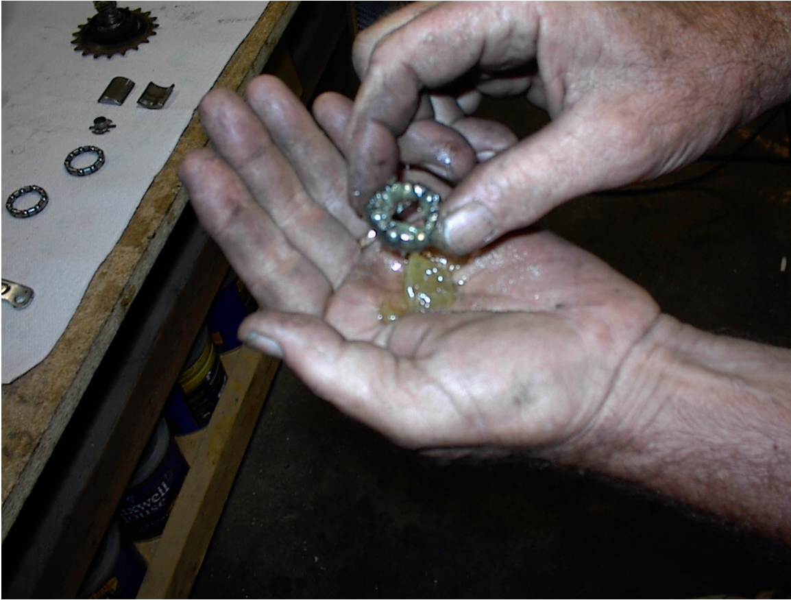
Fig. 18 Packing the bearings
