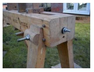
The best way to assemble this arrangement is shown in this picture. The bed is laid upside-down and the legs and bolts fed through the holes and tightened up before uprighting the lathe. Ignore the notches in the legs in the picture, these are from a previous experiment, however you should drilled a 12 mm hole near the basis of each leg so all the legs can be bolted together for transport, the picture of all the parts shows the legs bolted together.
