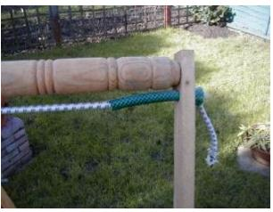
The top of these uprights are drilled 25 mm and a shoulder turned on the end of the spacer pole. No other fixing is required as the action of the bungee is to pull the uprights onto the spacer
