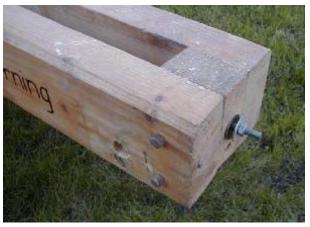
three pieces. A 18mm hole is drilled at each end of each side to accommodate the bolts that hold the legs in place. An 8 mm hole is drilled through the end of the spacer, this is for studding that holds the uprights for the bungee frame. Look at the pictures with the assembled legs and body to see the position of the holes. The edges of the bed are chamfered to make it easier to carry.
