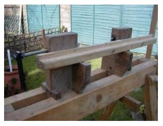
drilled straight through the poppet, for 12 mm studding this hole should be about 10 mm. To tap out the thread in the poppets file the thread at the end of the studying so it has a sharp step that will cut into the wood, use a brace to hold the threaded bar to tap through the studding. To help start the thread you can drill the outside end of a hole out to 12 mm diameter by about 20 mm deep.
