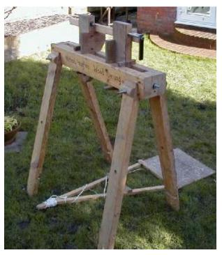
demonstrate, including the laying out of tools, wood and items for sale, is about 12 minutes. The time for assembly also makes this lathe suitable in an environment where the lathe is not left set up, for example, in an typical back garden.
