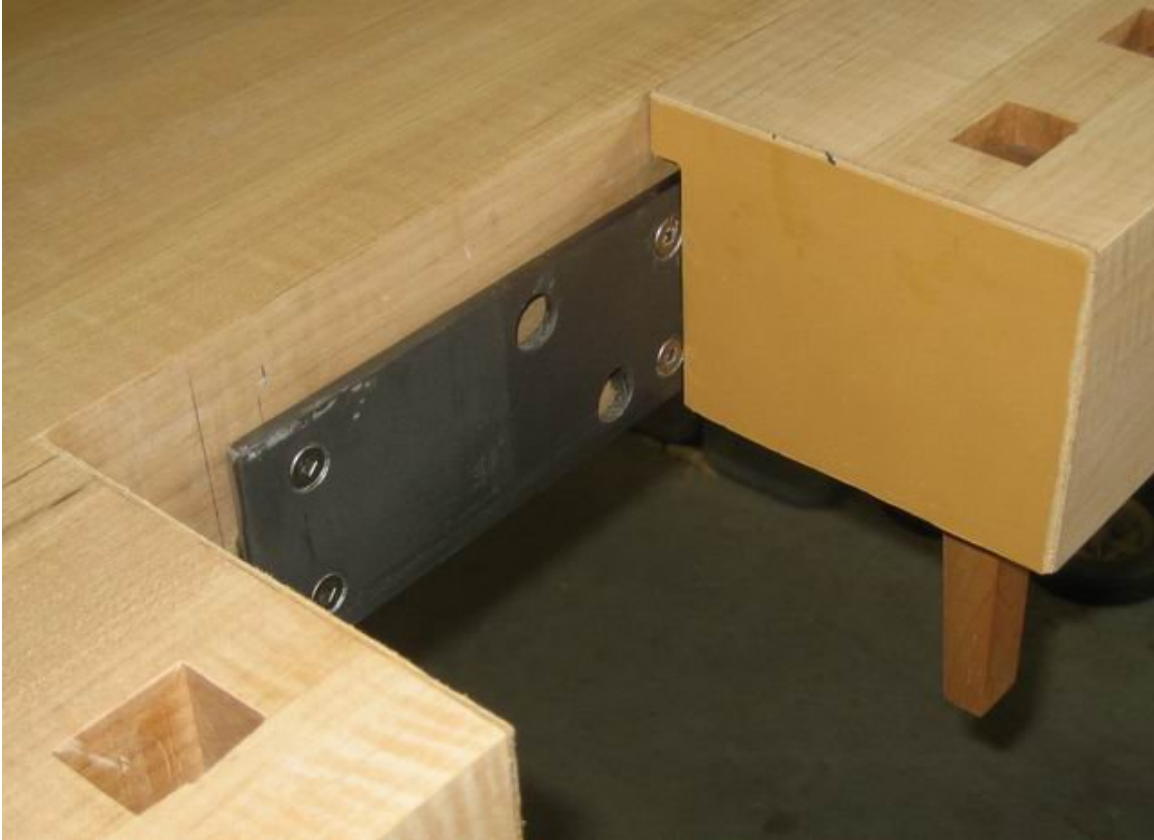
Figure 90: Tail vice jaw - lined with leather glued in place with 180 gram strength hide glue.
