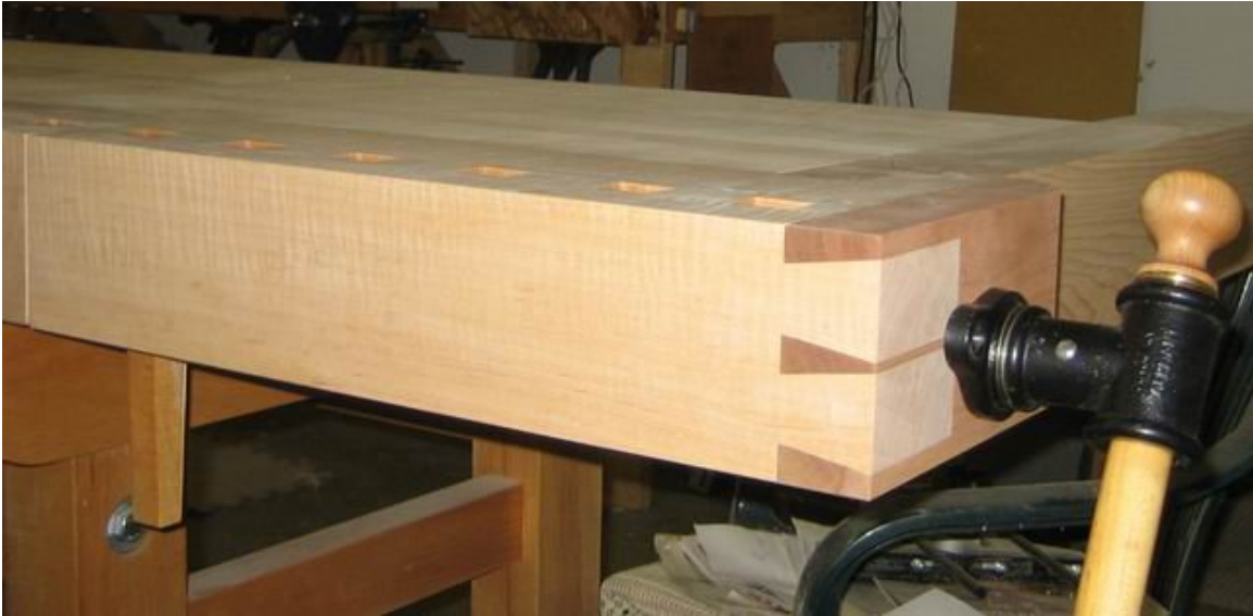
Figure 85: Finished tail vice (note undersized diameter handle) – March 13, 2006
