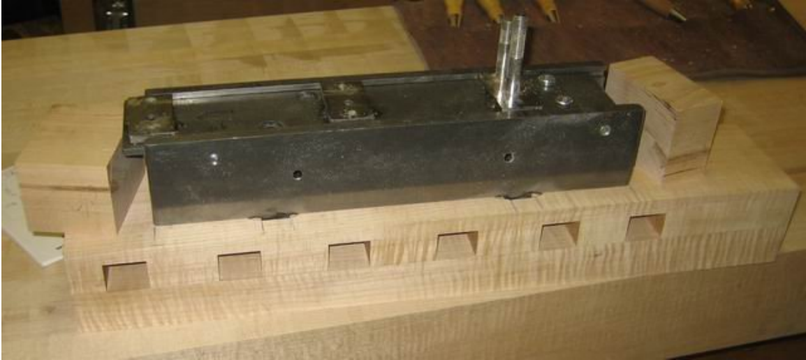
Figure 81: Tail vice assembly. Spacer blocks are glued to doghole strip. Then cover plate is glued on top of spacer blocks and is screwed to the welded assembly
