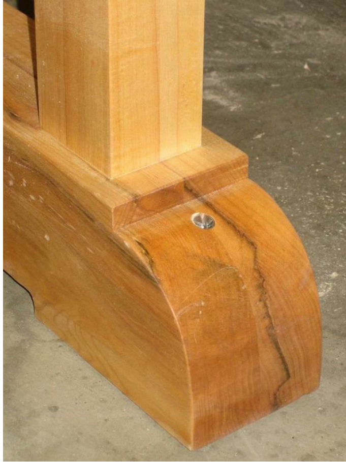
Figure 33: Completed foot showing leveller adjustment screw
