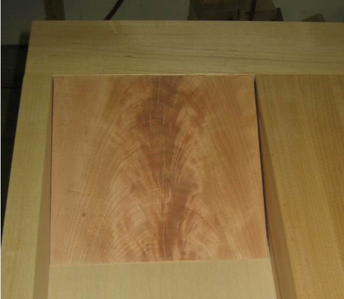
Figure 100: Finished tool tray ramp with cherry crotch veneer (approximately 1/8" gap allowed between plywood part of the tool tray ramp and the workbench to allow for expansion/contraction)
