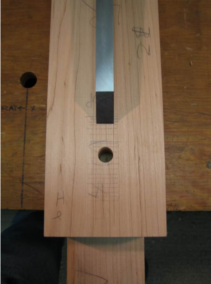
Figure 22: Chopping Mortises - drilling pilot hole
