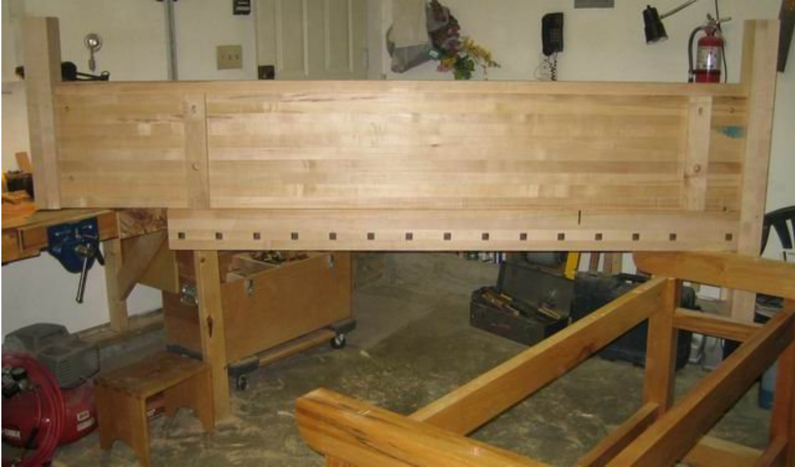
Figure 59: End-caps in place. Benchtop is getting very heavy. I had to turn the benchtop 180°. With only one person, it was a difficult task.
