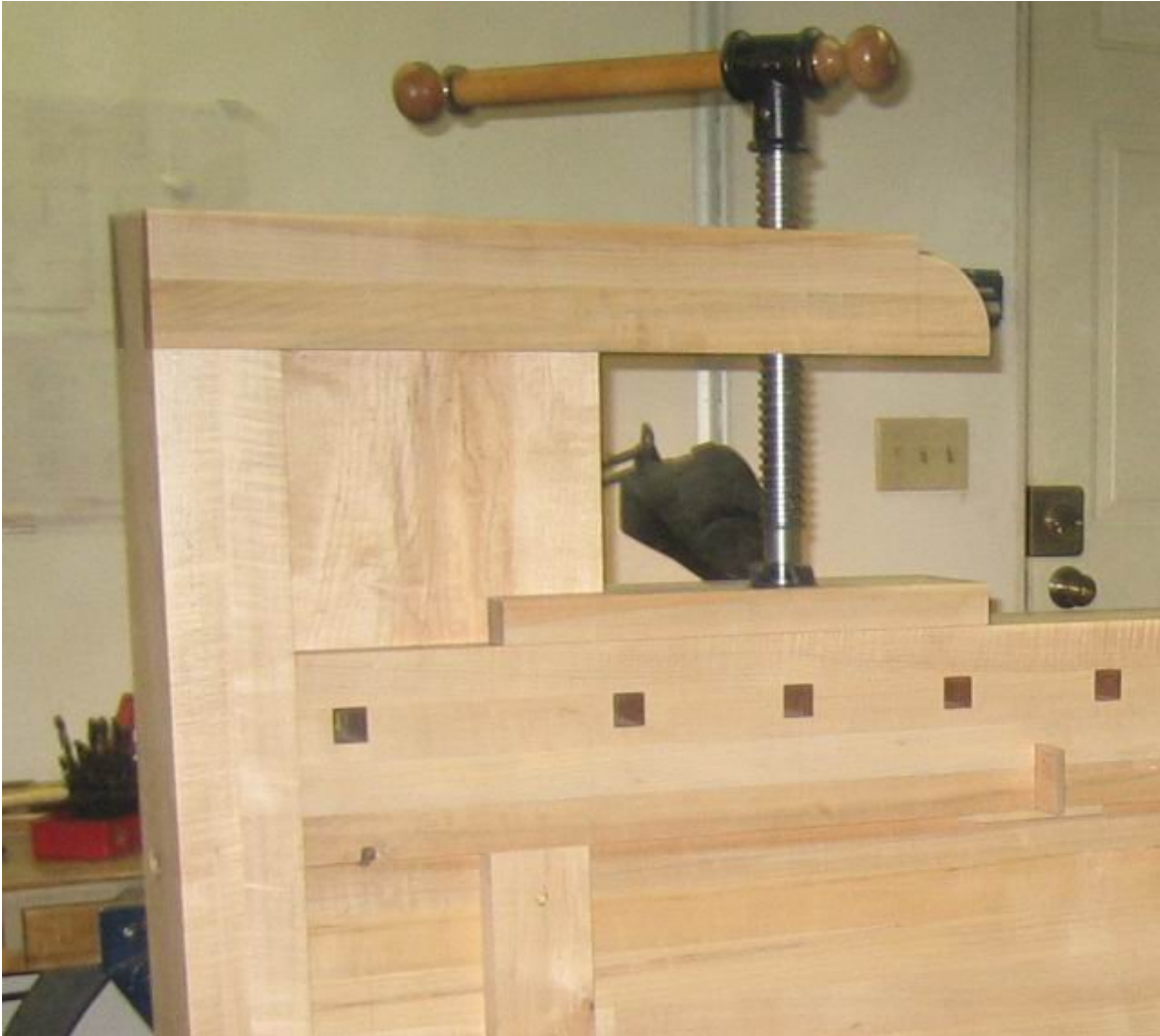
Figure 67: Underside of shoulder vice showing vice jaw and arm riding under the spacer block. Spacer block is allowed to expand/contract to the right side of the picture. Splines on left side of spacer block are glued.
