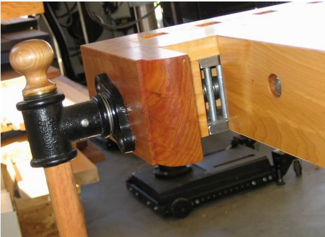
Figure 9: Tail vice end-cap and rear-view
