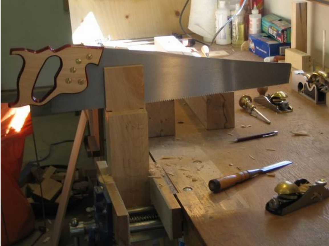
Figure 26: Finishing off the tenons with a handsaw
