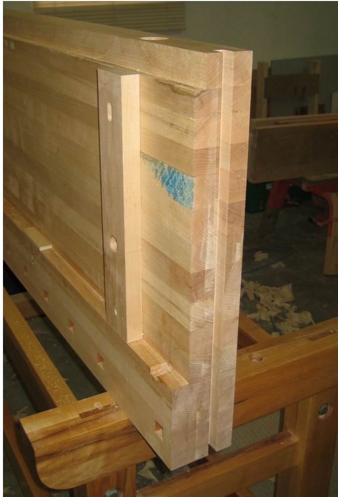
Figure 56: Spline groove formed in bench end – February 04, 2006
