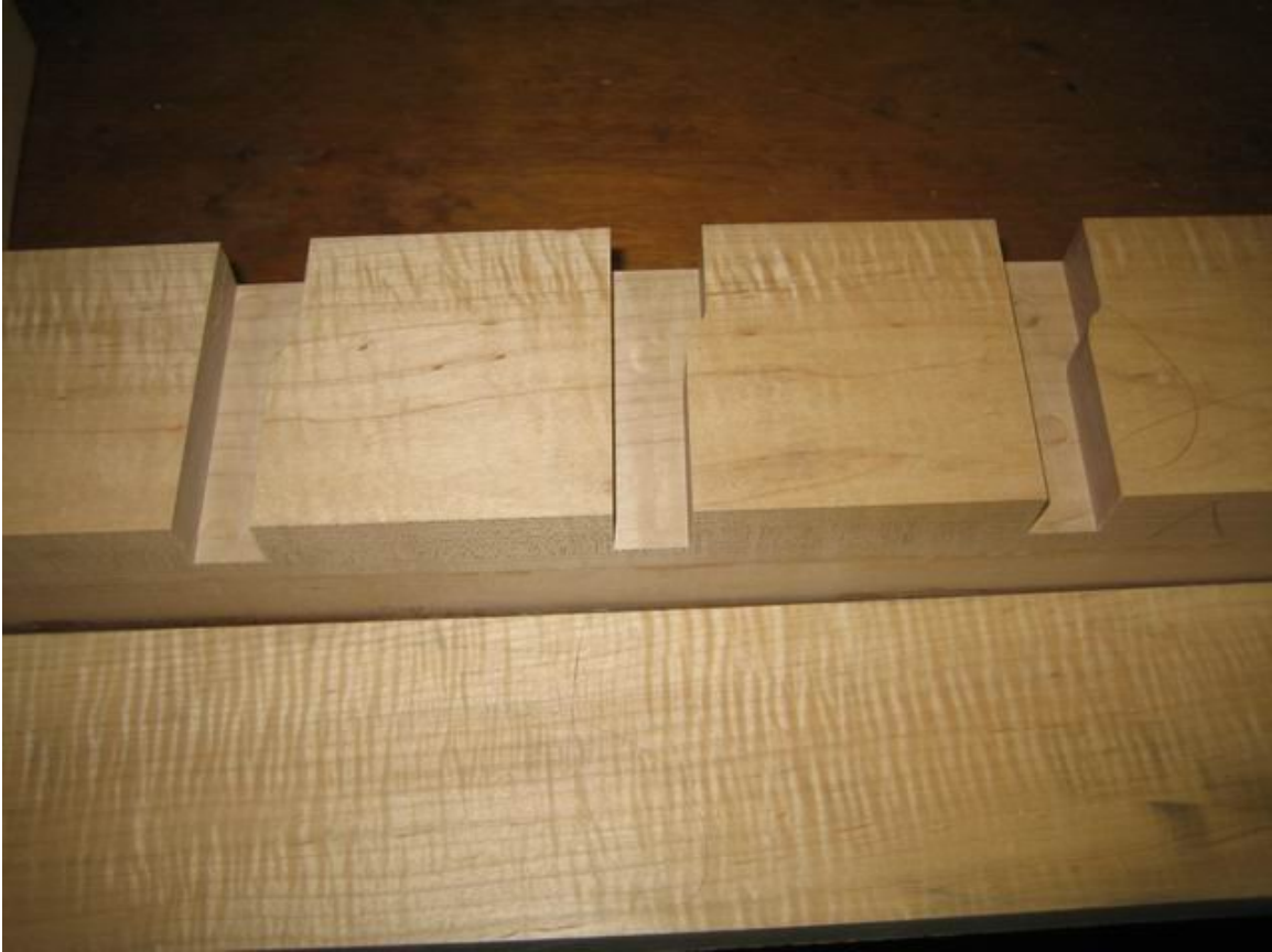
Figure 50: View of dogholes before cover strip glued on
