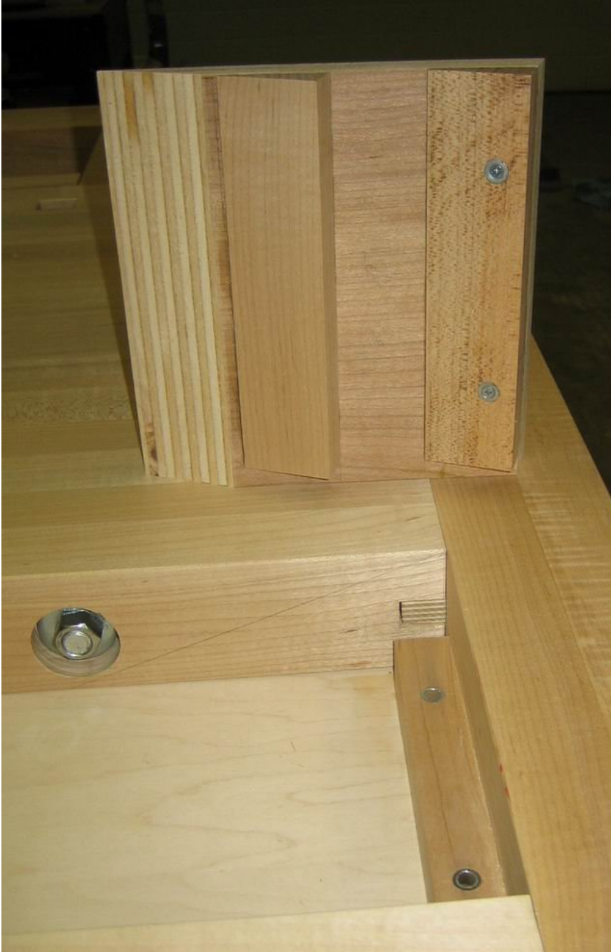
Figure 99: Tool tray ramp magnets (square block is glued to end-cap)
