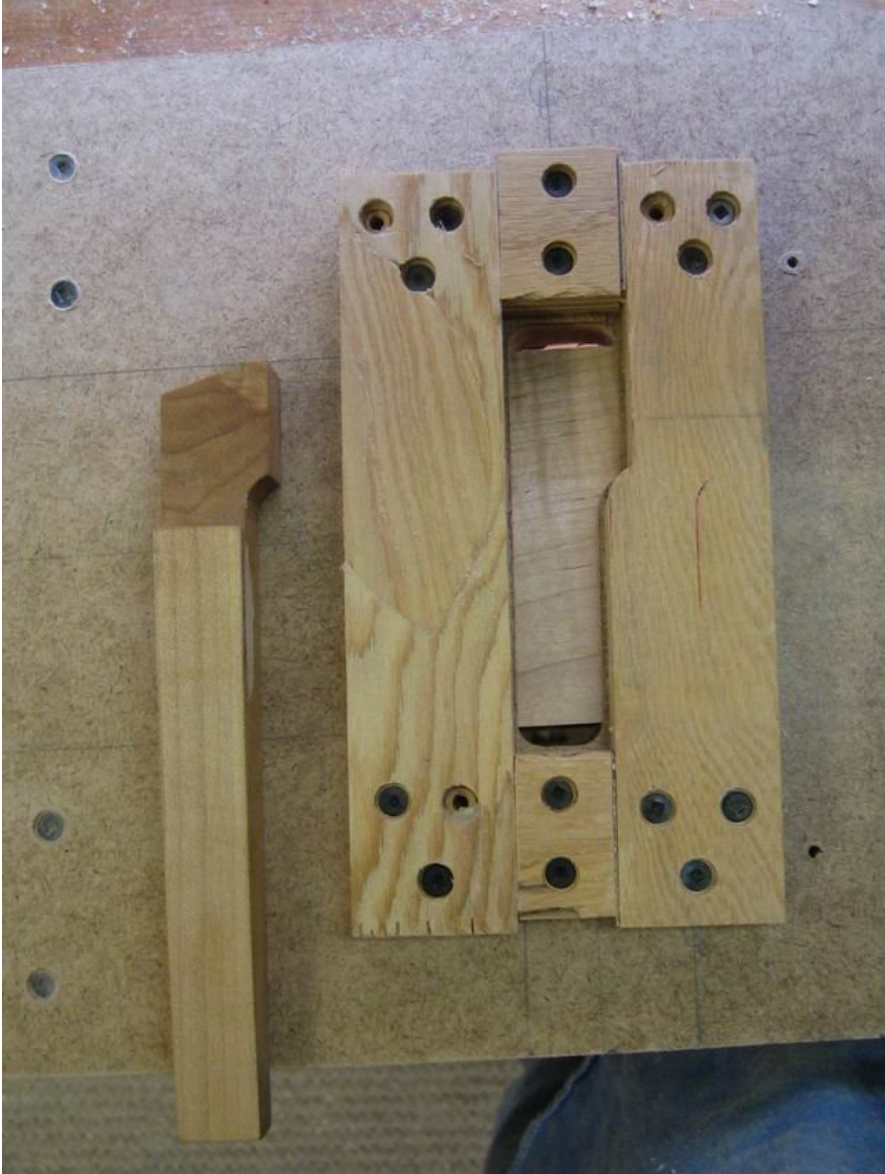
Figure 46: Benchdog and benchdog router template – top view
