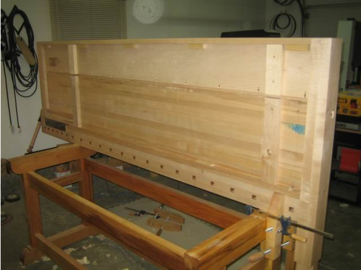
Figure 96: Underside of bench showing tool tray bottom, glue blocks, slotted screw holes, and spacer blocks
