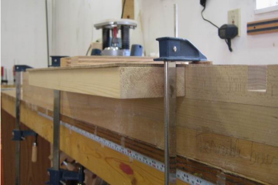
Figure 47: Benchdog template clamped in place – underside view showing one of the 2x4 guides
