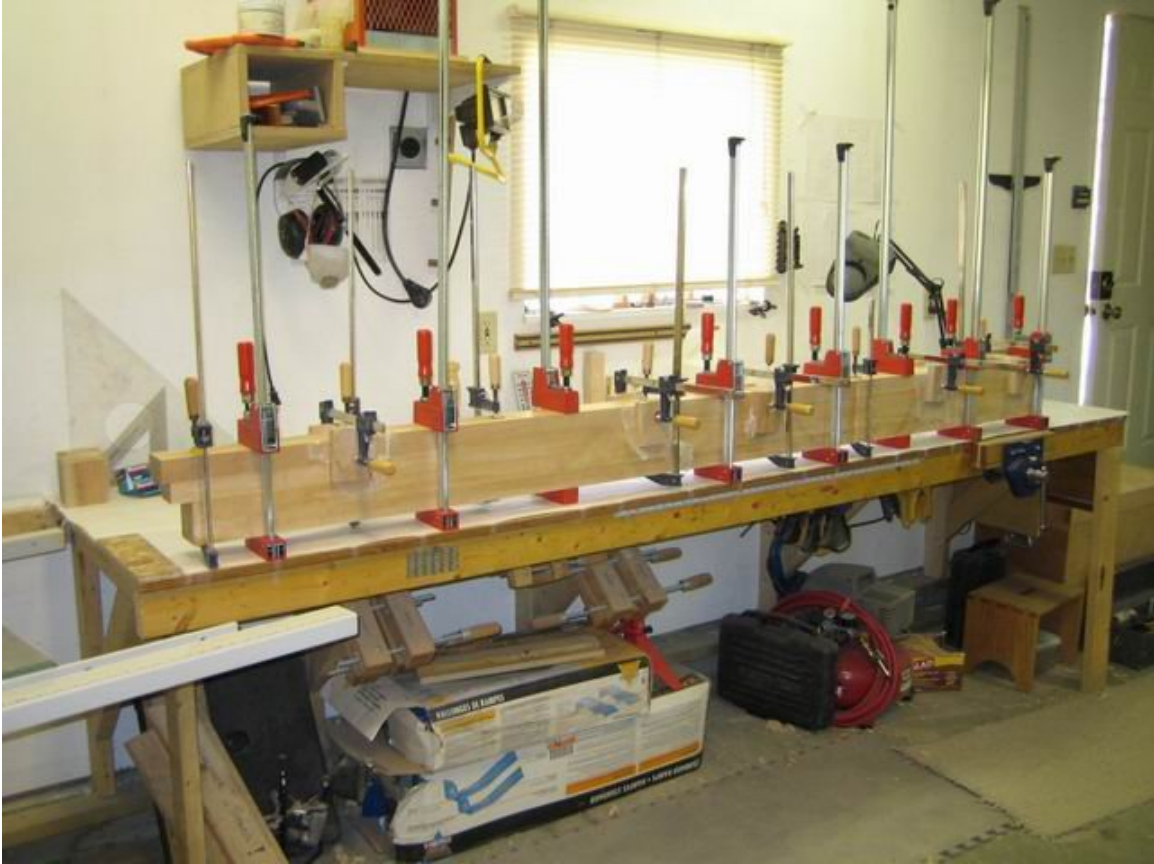
Figure 42: Gluing up the first course of four boards – May 29, 2005
