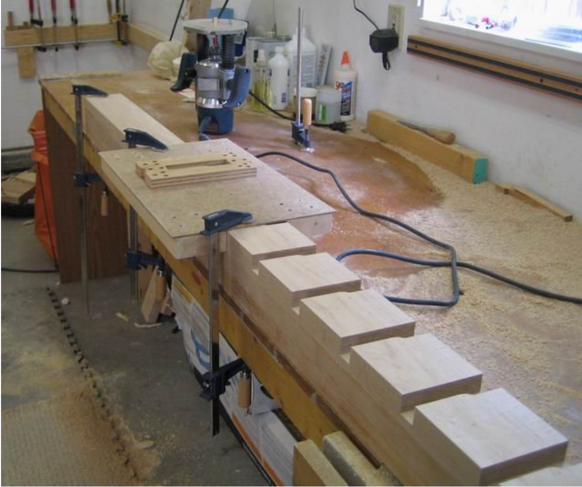
Figure 48: Routing benchdog holes – September 04, 2005
