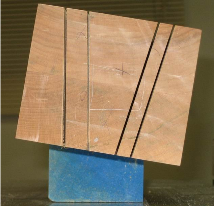
Figure 63: Cutting the shoulder vice pin-board on the bandsaw using an angled guide. Inside cuts were practice cuts. Outside cuts were cut very close to the line on bandsaw, then were cleaned up with a #60-1/2 rabbet plane.
