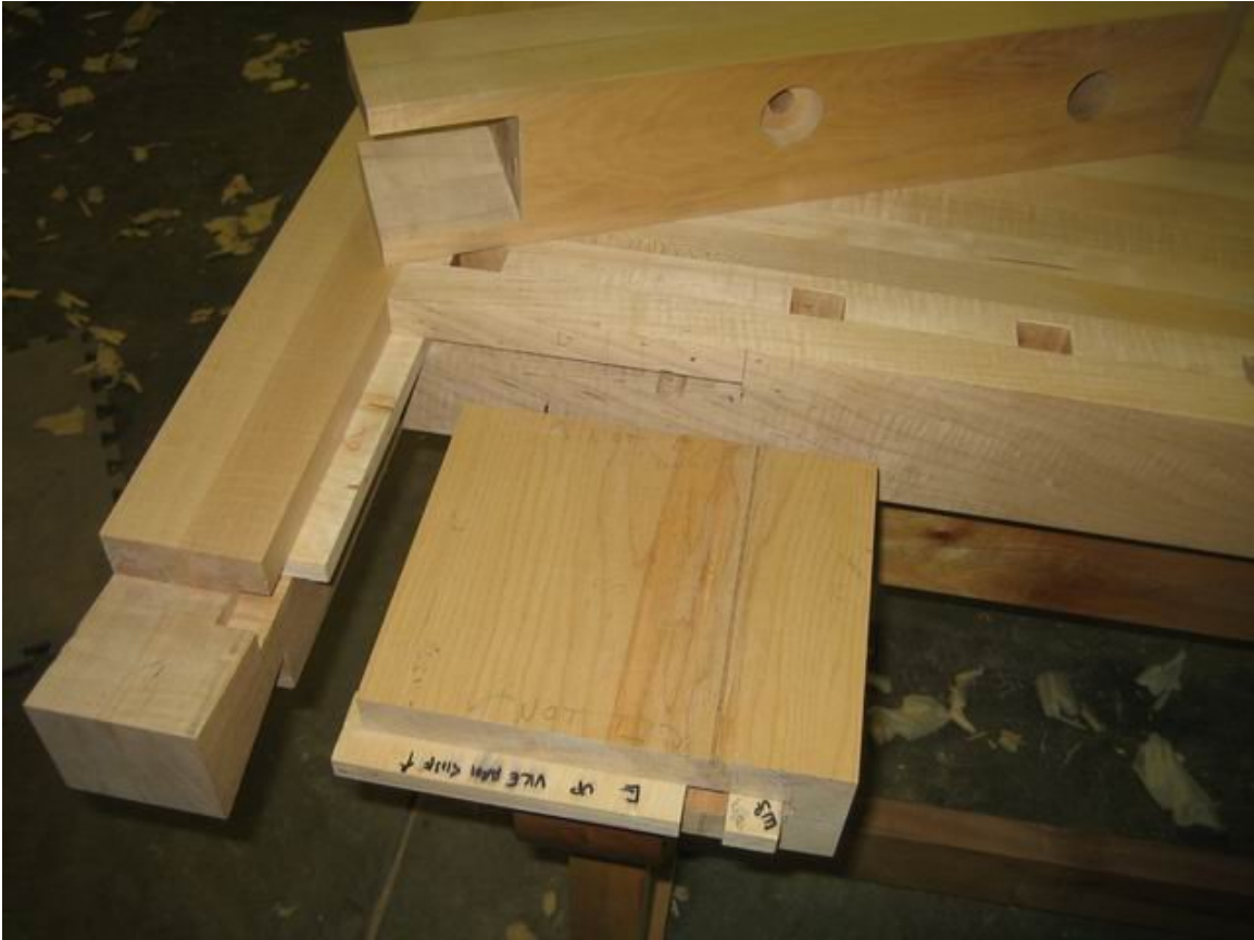
Figure 65: Exploded view of the shoulder vice
