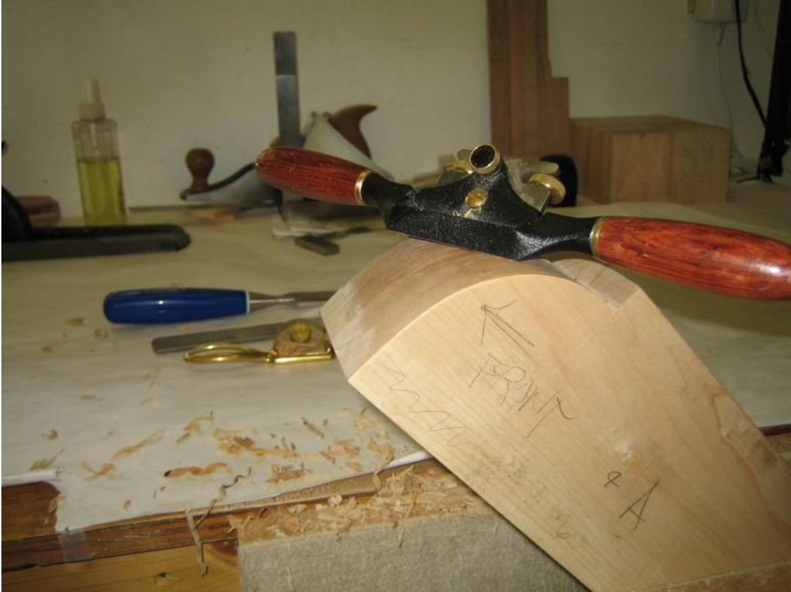
Figure 32: Final shaping of ends of sled feet
