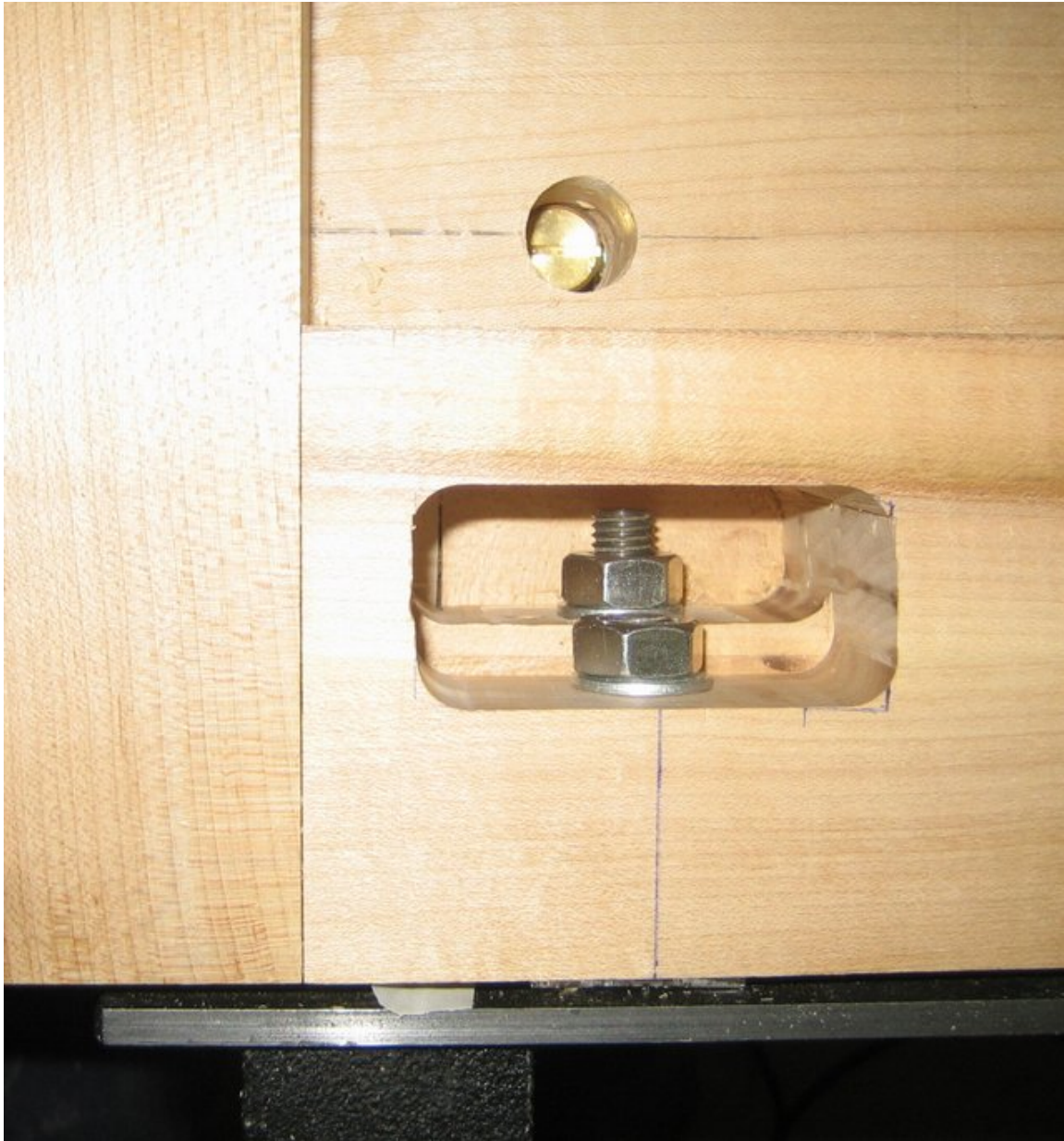
Figure 80: Underside view of mounting bolts (mounting plate visible at bottom of picture). The brass nut visible at the top is one of the bed-bolts holding the end-cap in place.
