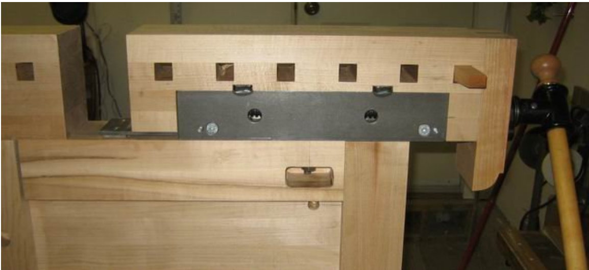
Figure 86: Underside of tail vice - partially open position
