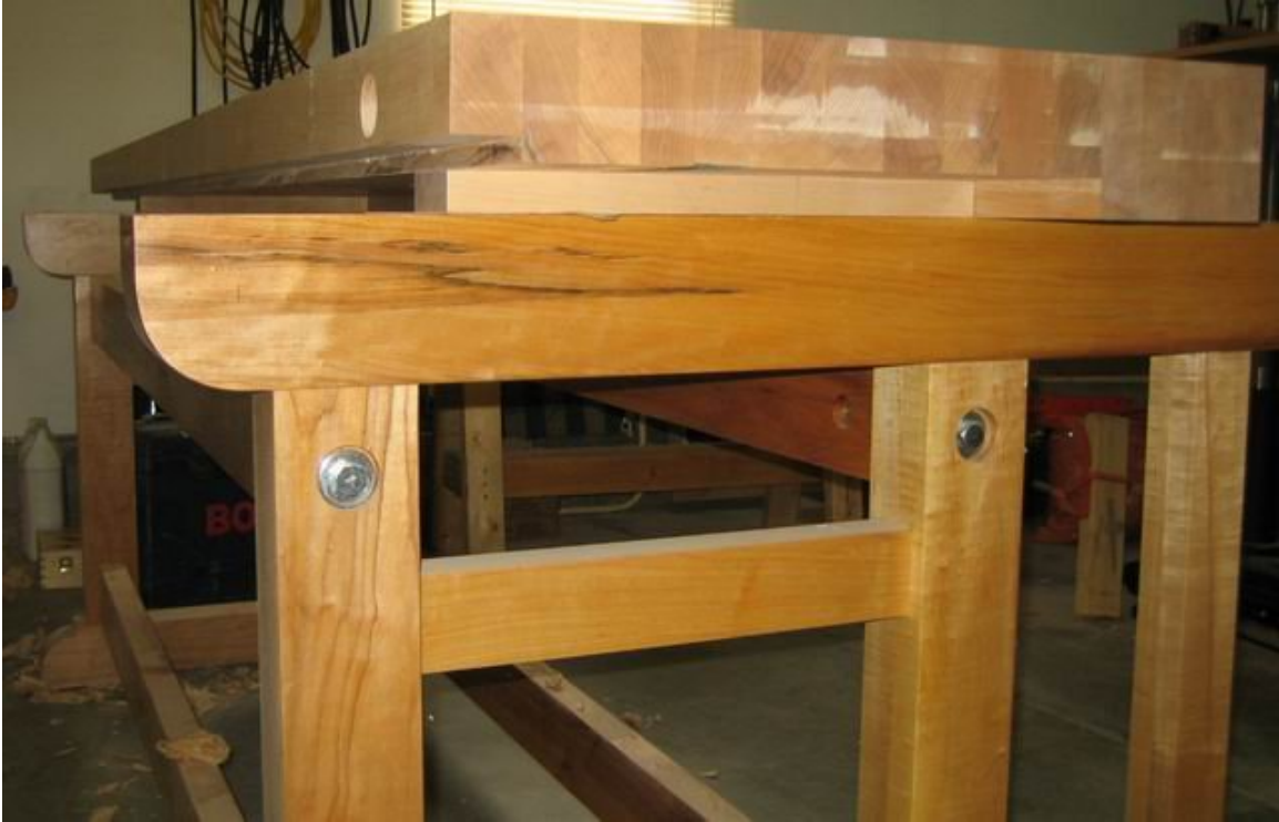
Figure 53: Doghole strip glue to main body of bench place. Filler strips under the 3" thick section of the bench are in place. Hole for shoulder vice threaded rod is visible at back of benchtop. November 27, 2005
