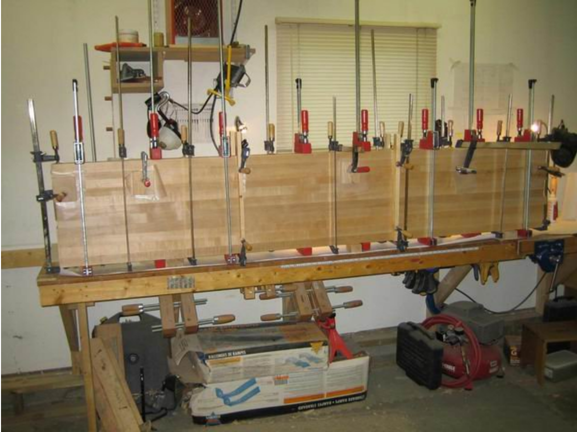
Figure 44: 3" thick part of benchtop being glued up – June 19, 2005
