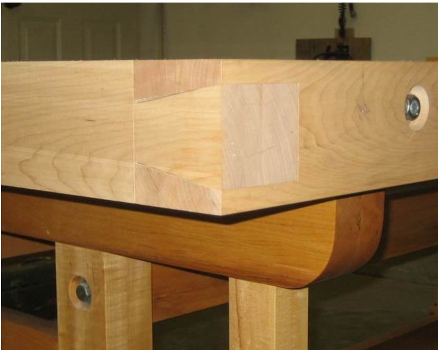
Figure 64: Assembled shoulder vice dovetail before glue-up
