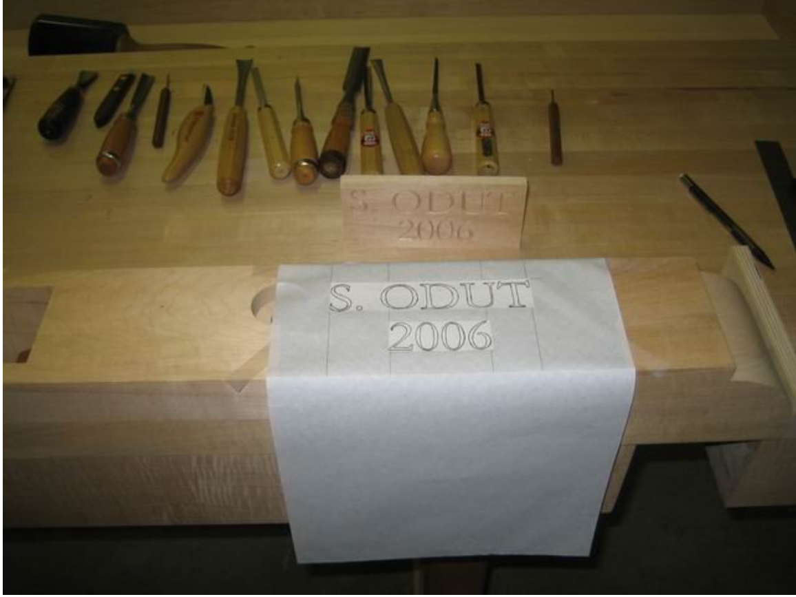
Figure 69: Transferring the lettering to the wood using carbon paper – practice piece in basswood is visible above the vice arm.
