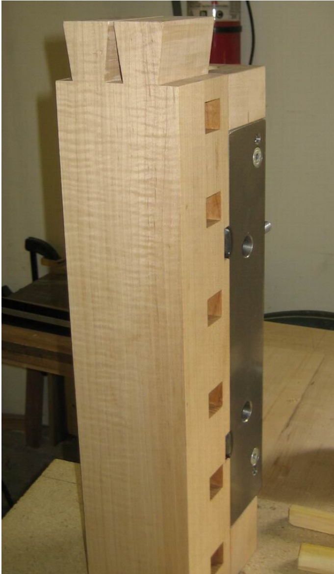
Figure 83: Dovetails cut for the tail vice assembly end-cap
