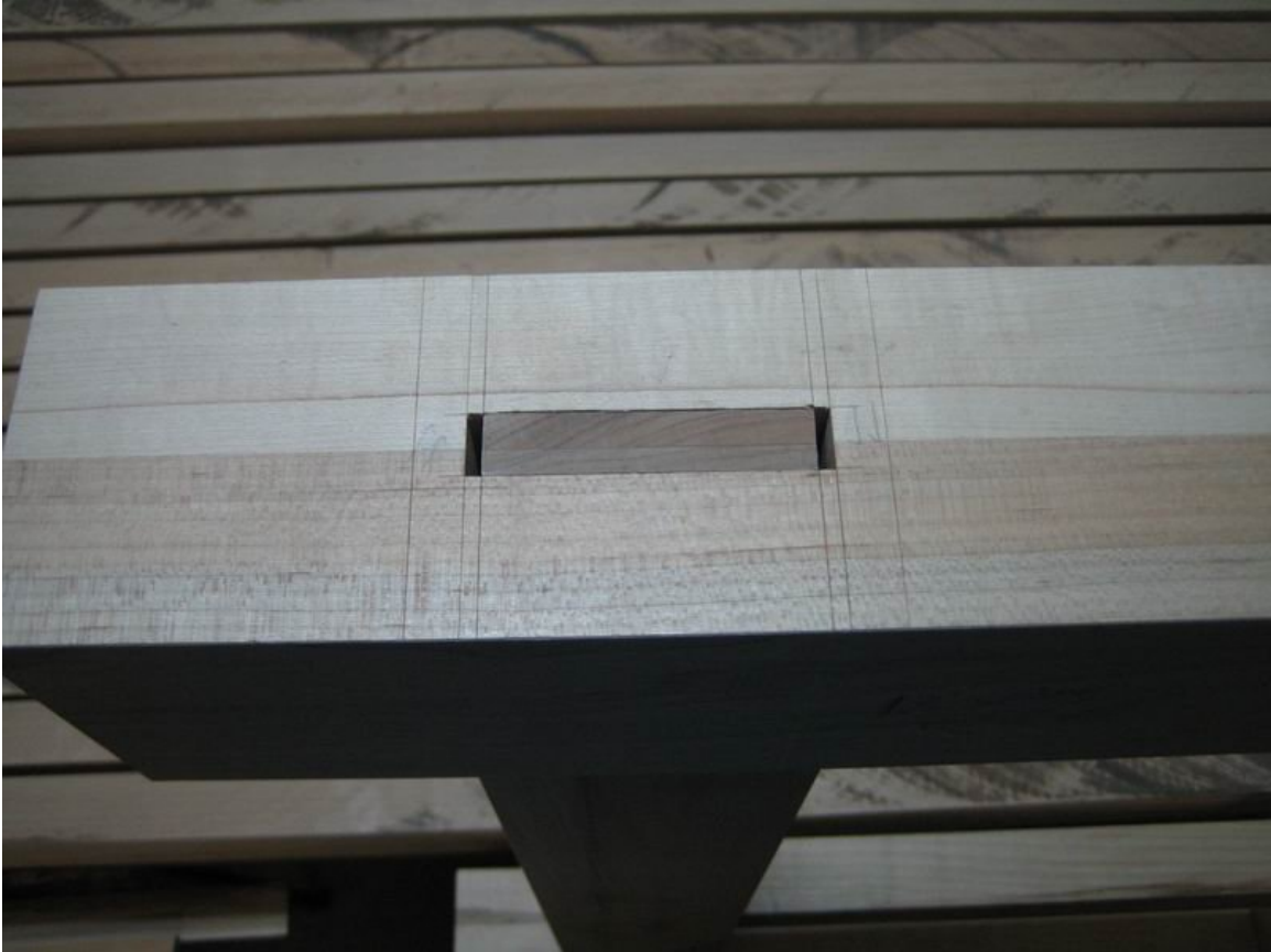
Figure 27: Through tenon - showing allowance in mortise for wedges
