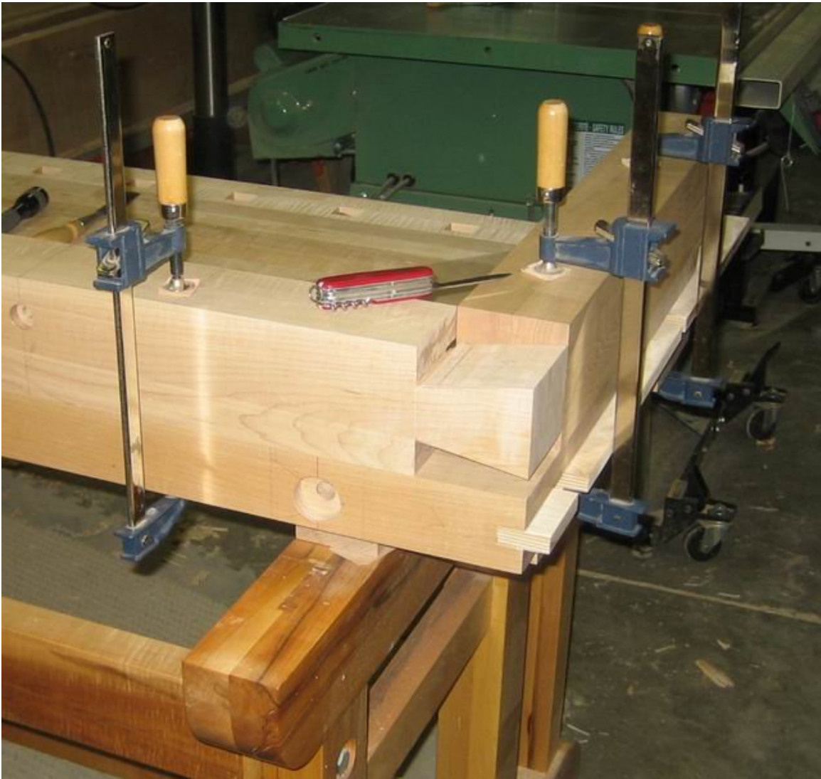
Figure 62: Transferring dovetail markings onto pin board
