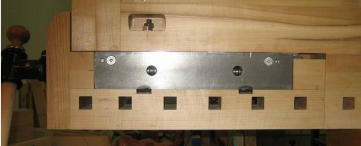
Figure 87: Underside of tail vice - closed position. Note that the jaws close very tightly to each other. By ensuring that the ends of the tail vice and the dog-hole strip were perfectly square before glue-up and assembly of the vice the jaws fit perfectly and I did not have to make any corrections.
