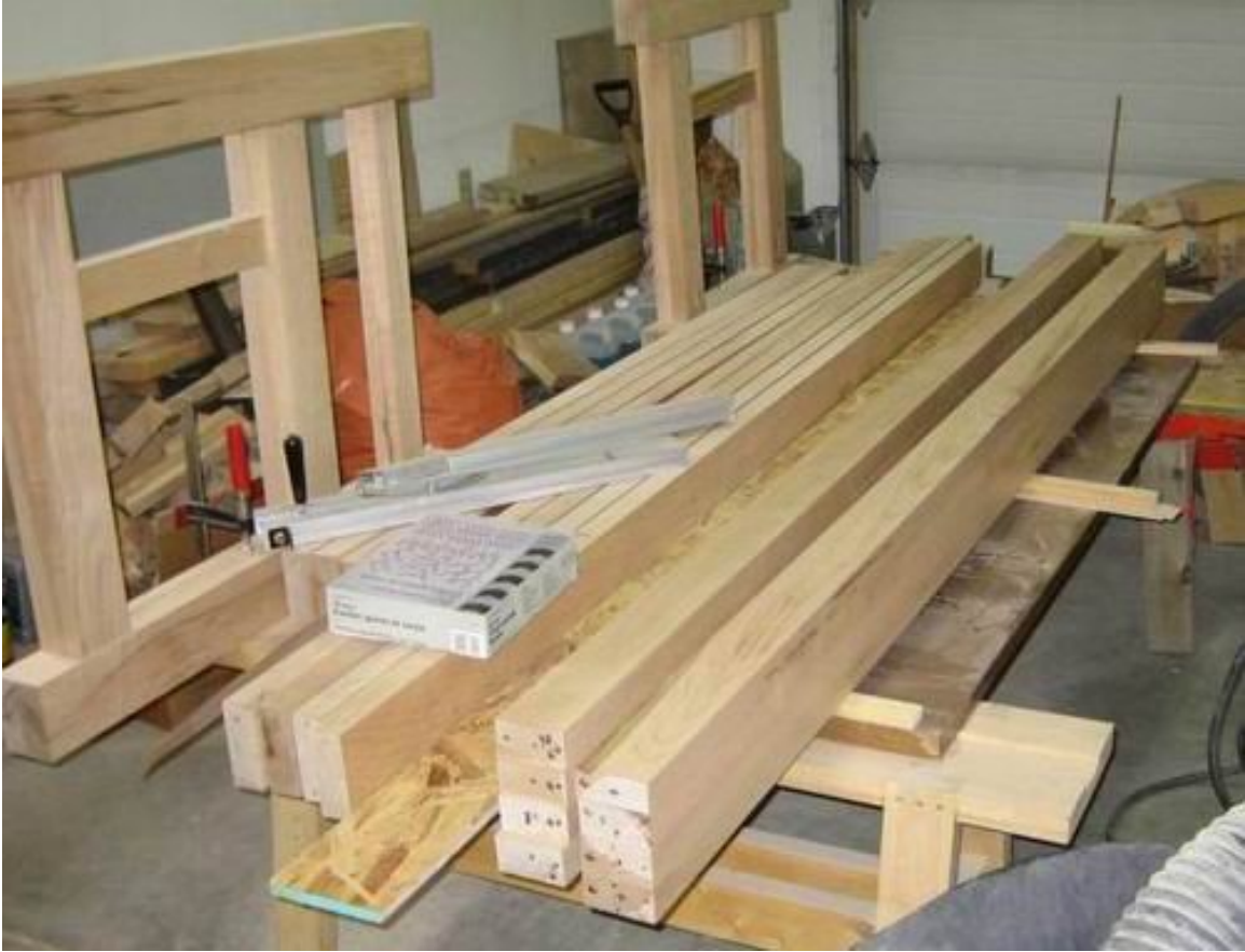
Figure 43: Two courses glued up and waiting – June 12, 2005
