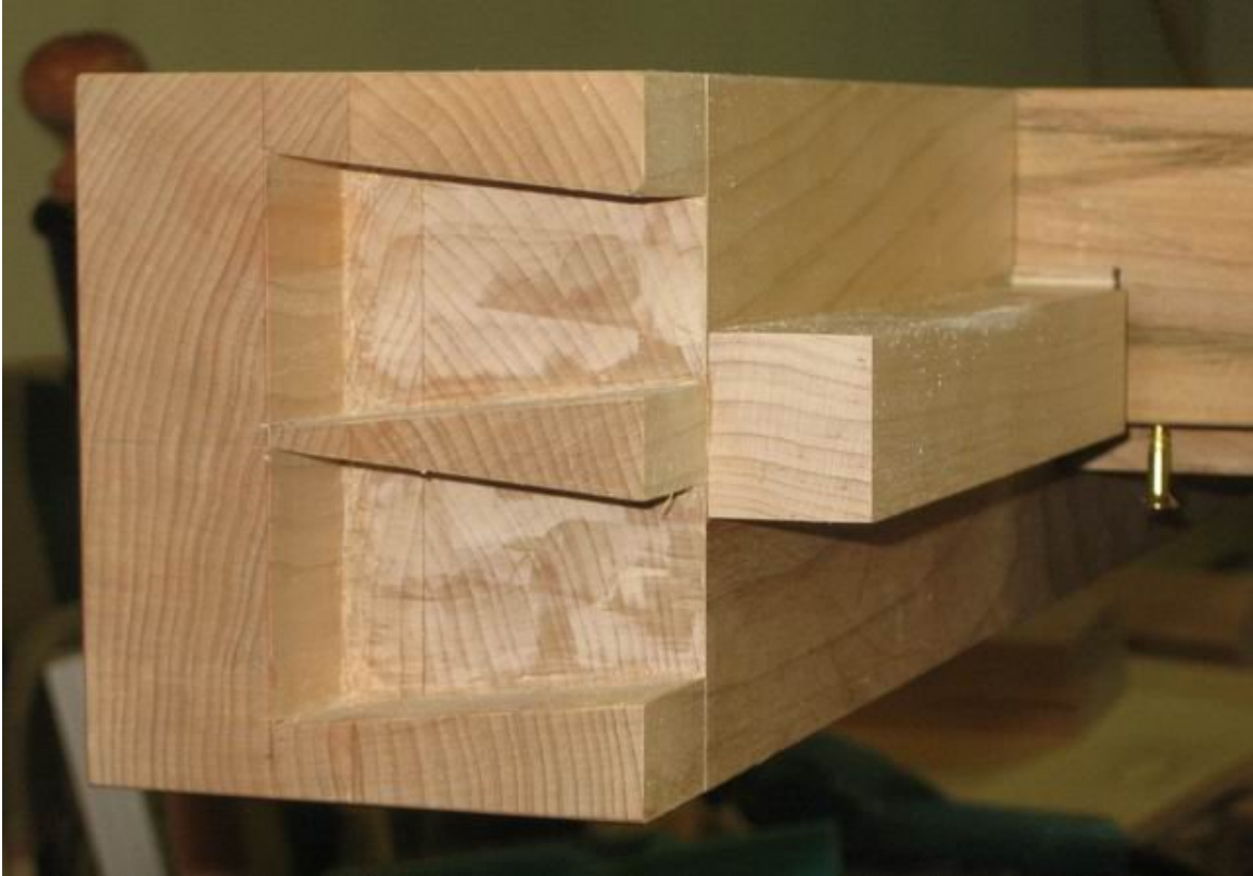
Figure 94: End-cap pins (glue block is to support the tool-tray ramp). Note the slight shavings taken off the inside face of the pins. This was done to get an exact fit between the back-board dovetail baseline distance and the exact distance between the two end-caps. Don't break off a corner of a pin when taking the shavings off (like I did).
