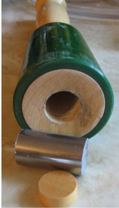
Figure 34: Broken mallet - doesn't pay to buy cheap (or at least you shouldn't pound on a cheap mallet too hard).
