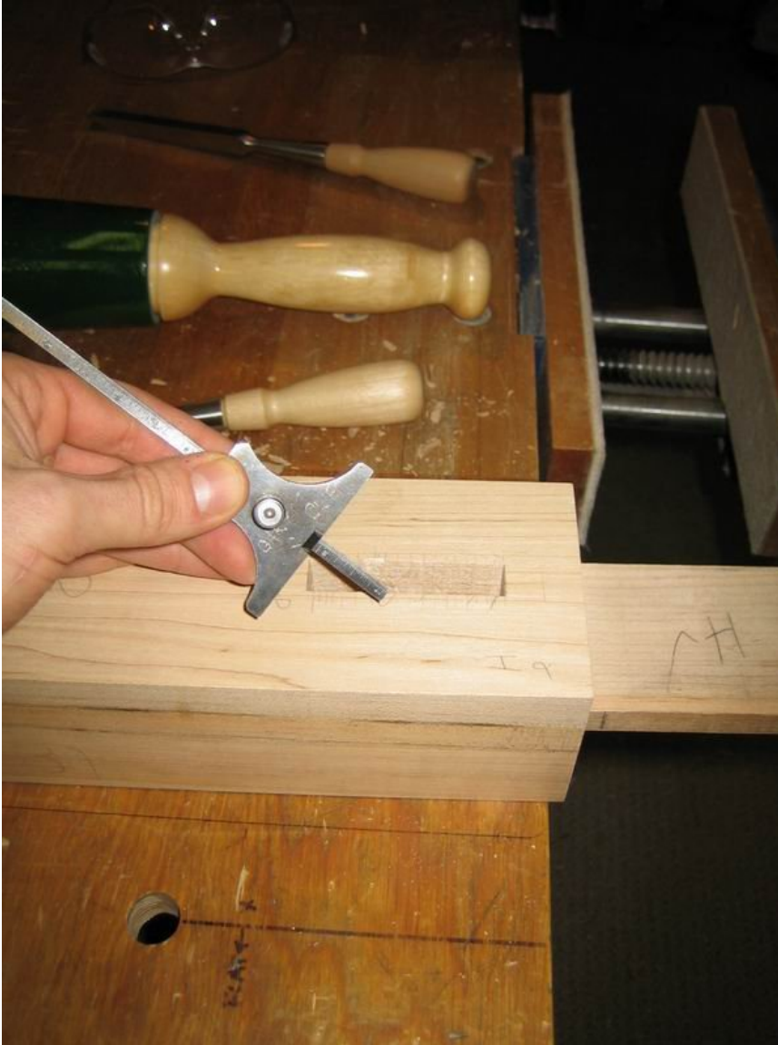
Figure 24: Chopping mortises - checking to see if ends and sides are square
