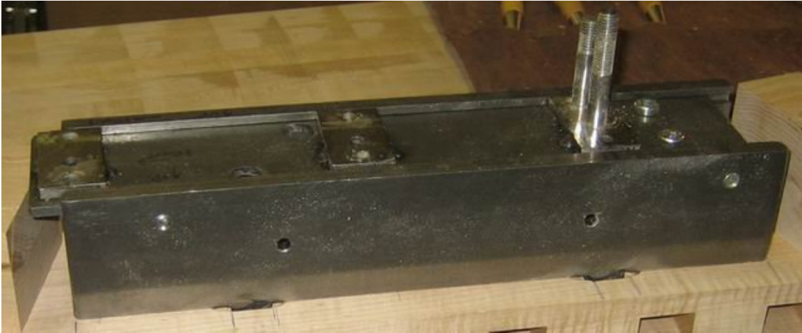
Figure 74: Small welded tail vice hardware - view from backside (note I modified one of the bolts to be shorter than the other bolt). Handle end of the vice is to the right and upper side of vice is in foreground of picture.
