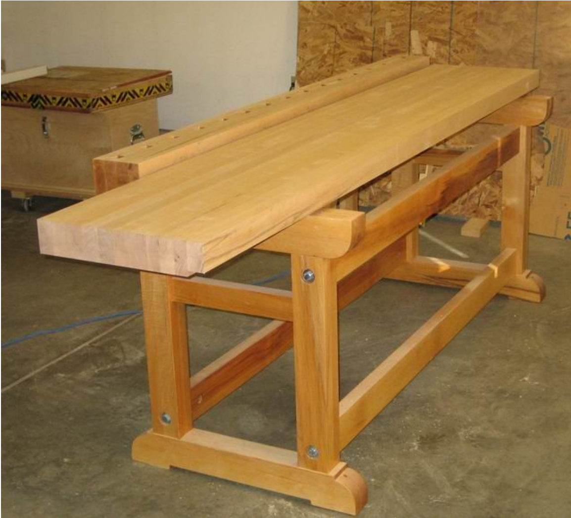
Figure 52: Benchtop before doghole strip glued in place (view from rear of bench) – doghole strip is 4” thick, remainder of benchtop is 3” thick.
