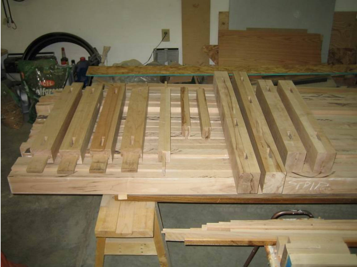
Figure 25: Chopping mortises – done!
