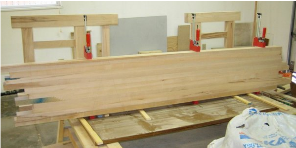
Figure 41: Benchtop boards laid out for best grain direction
