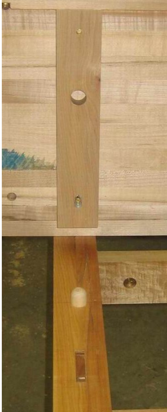
Figure 55: Underside of bench showing filler strip and bullet dowel
