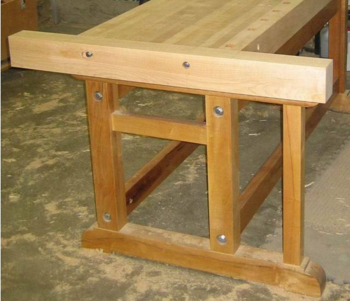
Figure 60: Shoulder vice end end-cap showing bed bolt locations. Bolt at rear of bench (to left) has a slotted hole to allow for bench expansion. Can you see the error in this picture? The yellow smudge to the left of the slotted bolt was an oops where I drilled the bolt hole in the wrong location. I plugged the hole, but it is slightly visible.
