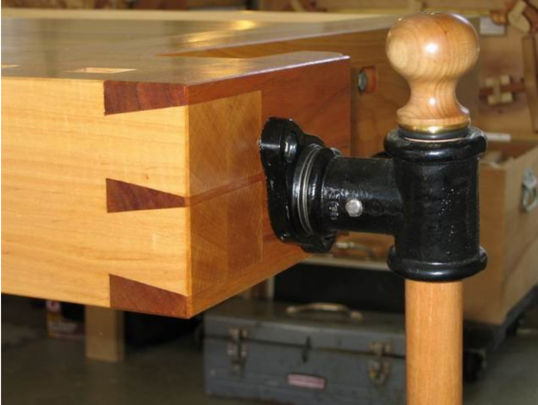
Figure 8: Tail vice dovetail and handle
